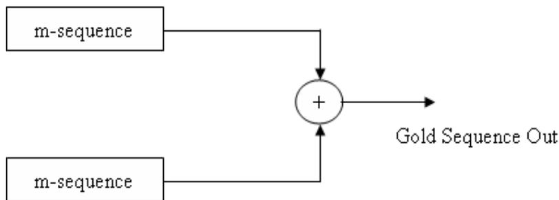
Figure 1. Block diagram of Gold code generator
